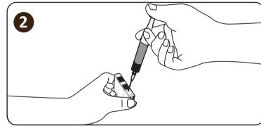
Fill the cartridge using a clean syringe and the corresponding color of Inkedibles Edible Ink through the refill port, and then replace the plug.
