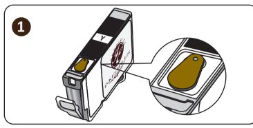
Before you refill your Inkedibles™ cartridge, you need to remove the sealing plug which covers the refill port.
