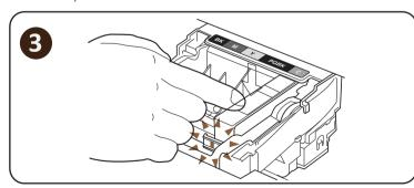
3. The cartridge is now ready to be installed into your printer. Make sure the cartridge "clicks" into place by pushing it down into its corresponding slot.
