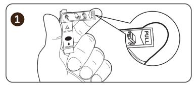
1. Remove the pull-tab on the top of the cartridge that says "PULL". This exposes a small breathing hole that the cartridge needs in order to print.
