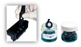
Place the seals in the jar with enough cleaning solution to cover them and allow the fluid to remove any ink residue.
