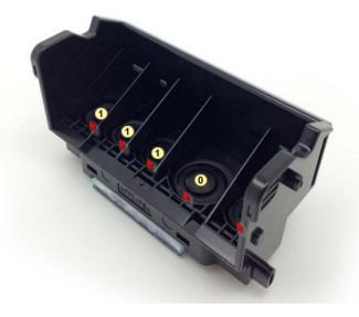
On the printhead, you will notice 3 or 4 smaller nozzle contact spots (indicated with the number #1 in the diagram). There is also a larger nozzle contact spot indicated with the number #0. Using a cotton swab or soft cloth, apply a small amount of cleaning solution to each contact spot and let soak for 3 minutes.
